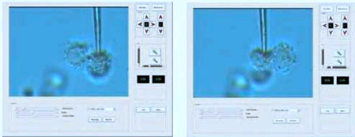
Figure 3. Screen shots of the injection process of single cells using the Hydro-MiNa robotic system.
