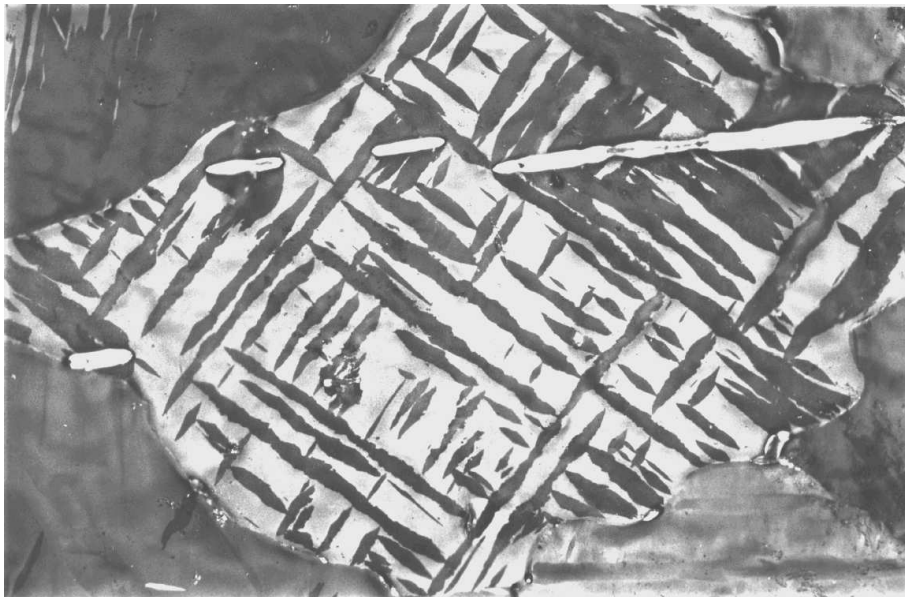
Figure 2: Twin network and four cleavage cracks in a large flat zinc grain coated on a steel sheet (grain size : 500\mu\text{m} ).
